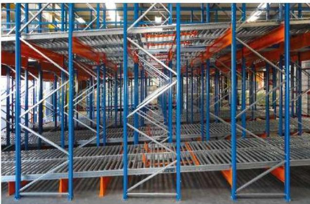
For order picking involving small packages with high turnover, flow racks have the advantage that they make buffers possible for the pick location.
