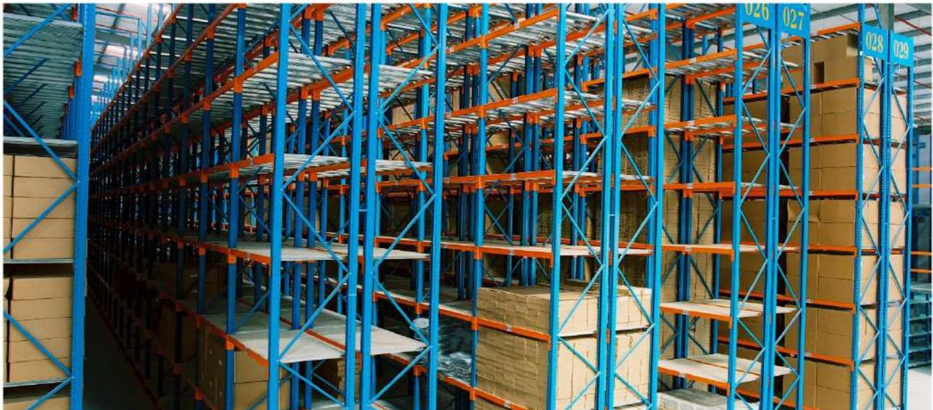
Long span shelving is a heavy duty hand loaded storage system that is designed to store large, heavy and bulky items. The step beams are designed to take 40mm thick chipboard and steel panels
